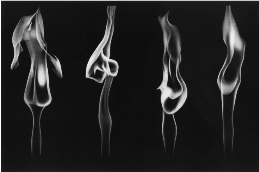
Fig. 1. Photograph of the ethylene diffusion flame at four successive time slices.
